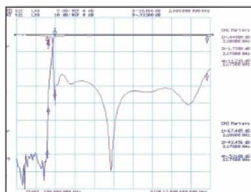
Typical plot of 2.6 to 13 GHz Highpass Filter
